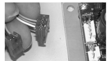
and let the board hang on the outside of the box with the back of the board facing you. Disconnect both wire plugs from the back of the controller. Then plug the kiln back in. Apply power to kiln. If fuse blows, replace the transformer. (If the fuse does not blow, the problem is a board or relay. Go to step 2.)
