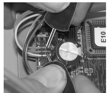
facing you. Plug the kiln back in. Touch voltmeter probes (in AC mode) to both INPUT connections (the white and orange wires).
